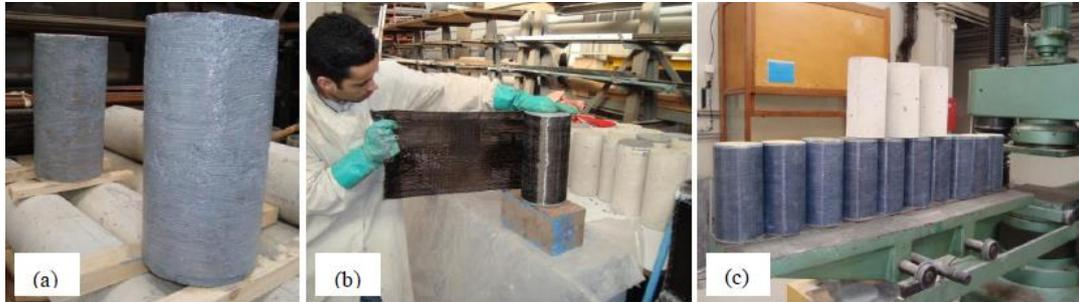
Fig. 4(a) application of primer adhesive; (b) application of CFRP wrap; (c) specimens wrapped with CFRP
