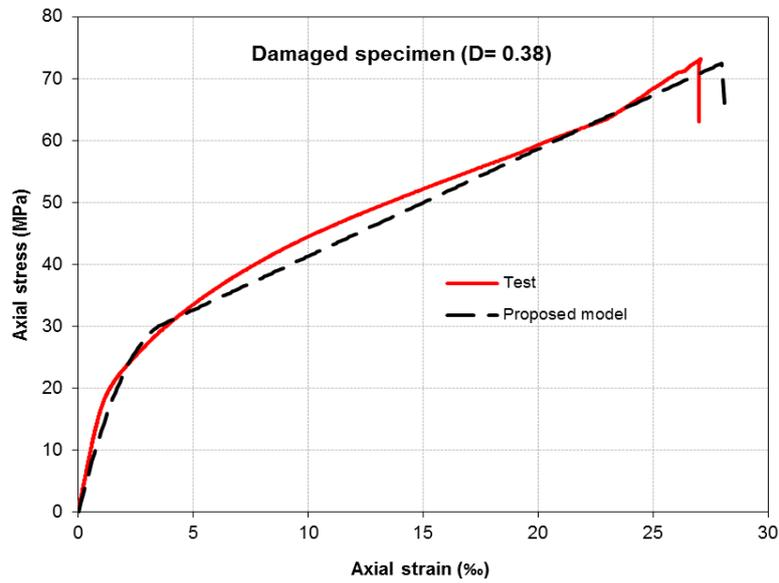
Fig. 14 Comparison of stress-strain curves of specimen D.R.S-80%-3L
