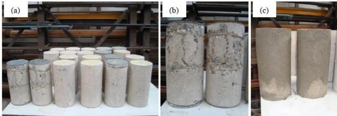
Fig. 3(a) Specimens after initial damage; (b) spalled cylinders; (c) mortar repaired cylinders
