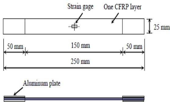
(a) Dimensions of CFRP flat coupons
