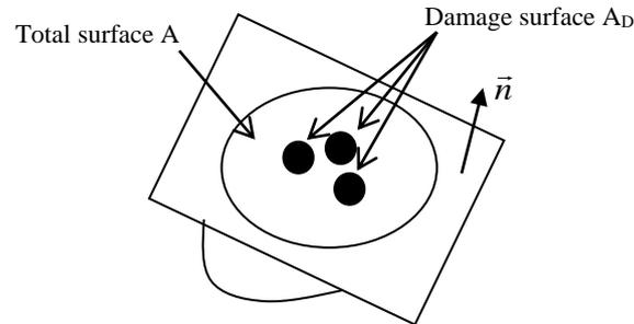
Fig. 9 Definition of damage (Comby 2006)
