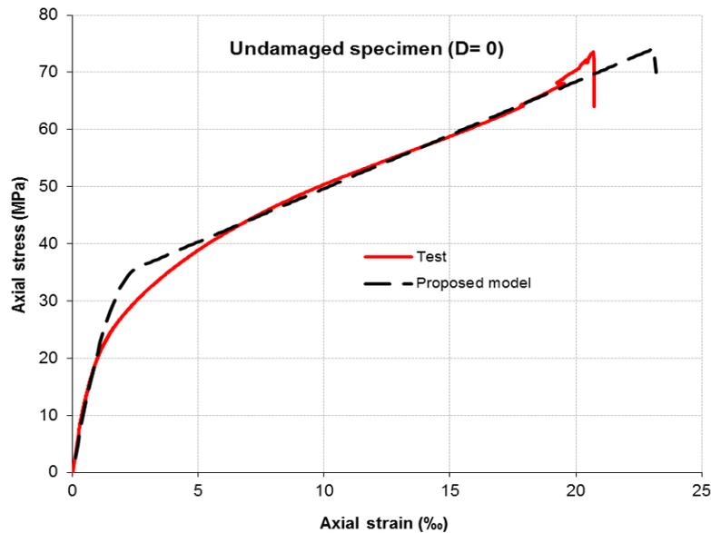
Fig. 11 Comparison of stress-strain curves of specimen S-0%-3L
