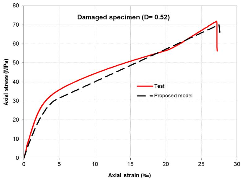
Fig. 15 Comparison of stress-strain curves of specimen D.R.S-100%-3L
