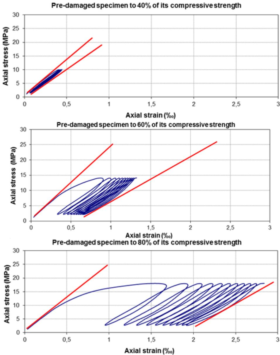
Fig. 2 Various damage situations with repeated compressive loadings (10 loading/unloading cycles)
