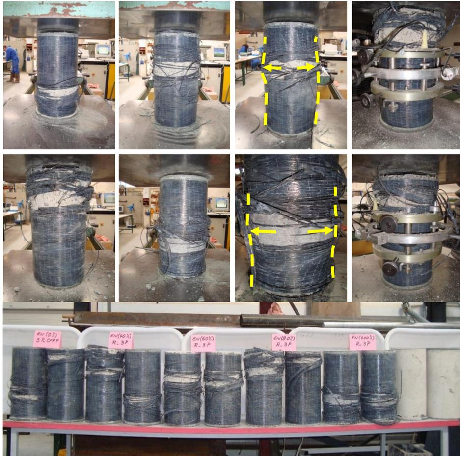
Fig. 8 Typical failure modes for some pre-damaged and undamaged strengthened specimens
