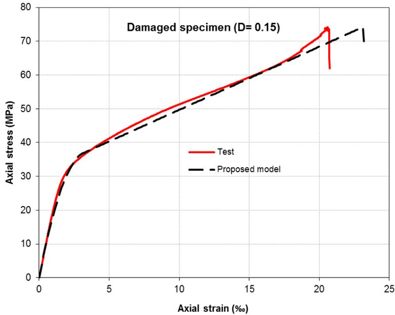
Fig. 12 Comparison of stress-strain curves of specimen D.R.S-40%-3L
