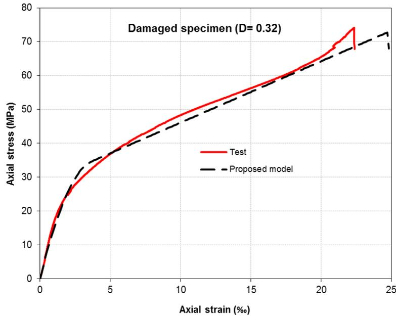
Fig. 13 Comparison of stress-strain curves of specimen D.R.S-60%-3L
