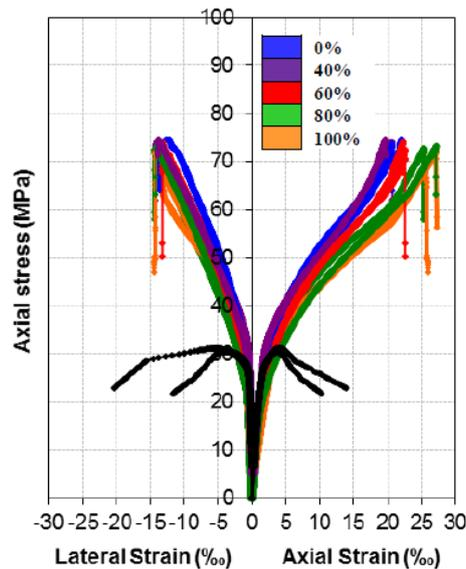
Fig. 6 Axial stress-axial and lateral strain curves for CFRP jacketed pre-damaged RC cylinders
