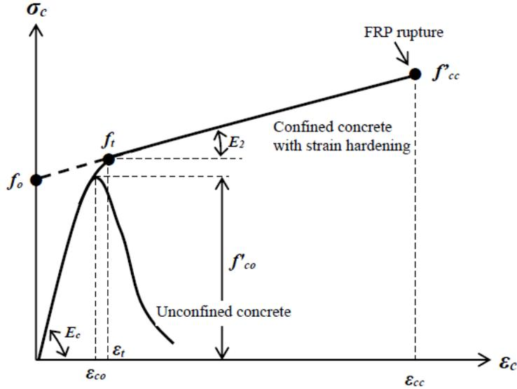
Fig. 10 Typical stress-strain responses and model parameters (Fahmy and Wu 2010)
