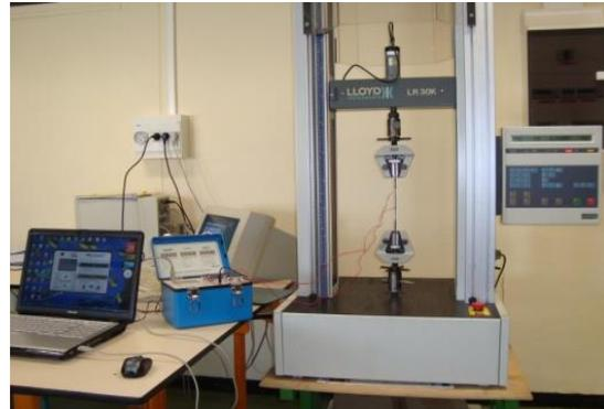
(b) CFRP specimen being tested in direct tension
