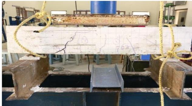
Fig. 5 Four-point-bending test on beam with final failure (due to shear cracking)
