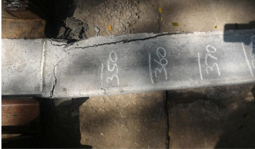
Fig. 7 Four-point-bending test on beam with final failure (due to shear cracking)
