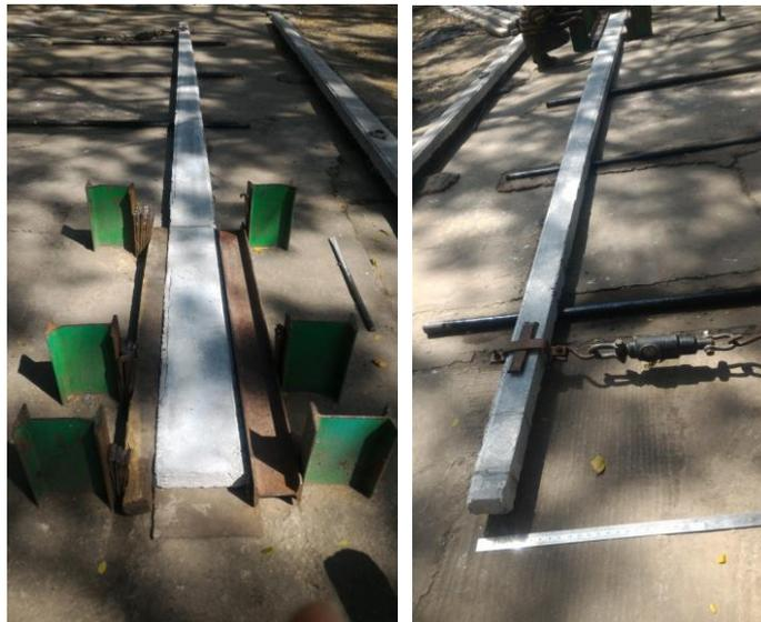
Fig. 6 Test set up for poles (with fixed bottom end and loading frame)
