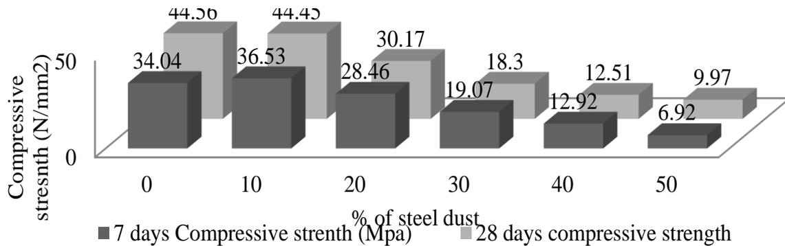
Fig. 8 Comparison between the compressive strength
