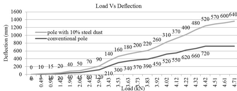
Fig. 10 Comparison between load vs. deflection curves for poles
