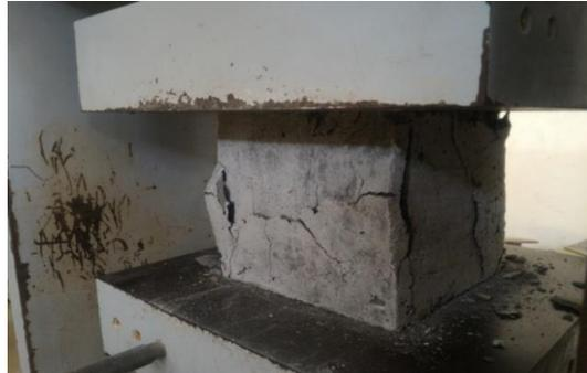
Fig. 4 Compression test on cube
