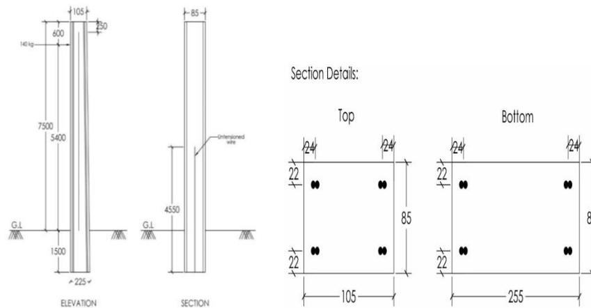
Fig. 3 Prestressing strand detailing for overhead poles
