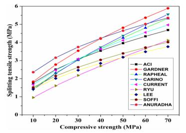
Fig. 9 Relationship between compressive and splitting tensile strength at 28 days
