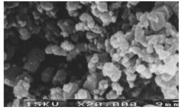
Fig. 1 SEM image of RHA particles
