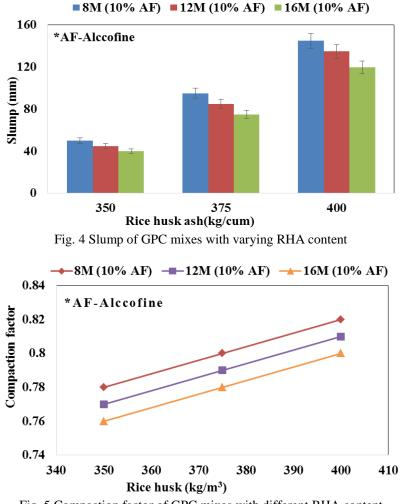
Fig. 5 Compaction factor of GPC mixes with different RHA content
