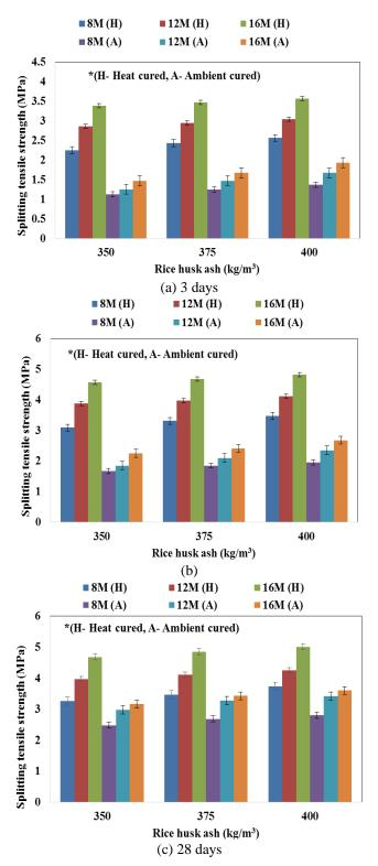
Fig. 7 Splitting tensile strength of RHA based GPC
