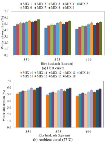
Fig. 8 Water absorption of RHA based GPC after 28 days
