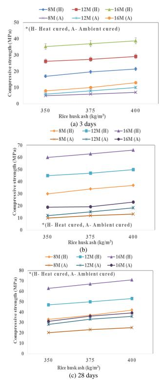
Fig. 6 Compressive strength of RHA based GPC
