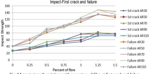
Fig. 8 Impact strength variations with percentage of fibre at first crack and failure
