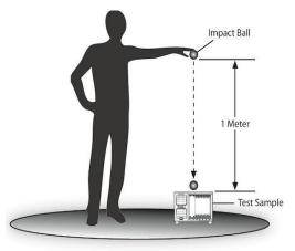
Fig. 4 Impact test
