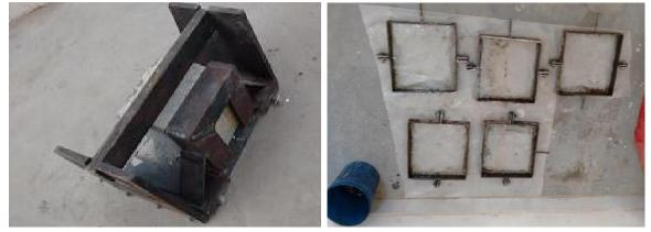
Fig. 2 L Shaped shear specimens
