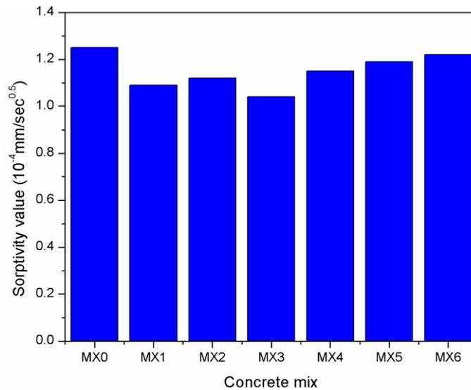
Fig. 6 Sorptivity of concrete at the curing ages of 28 days
