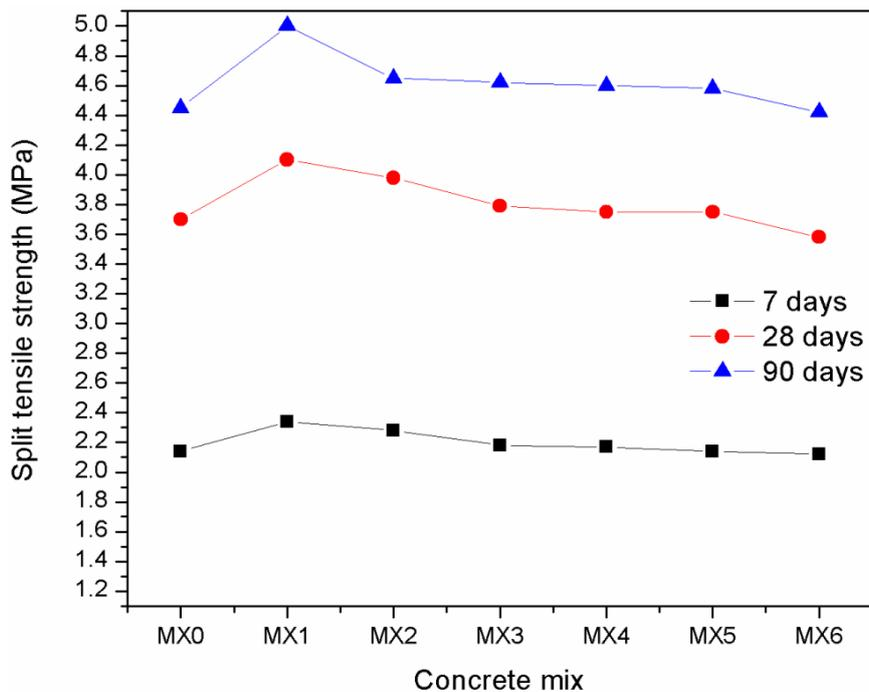
Fig. 2 Split tensile strength of concrete at the curing ages of 7, 28 &amp; 90 days
