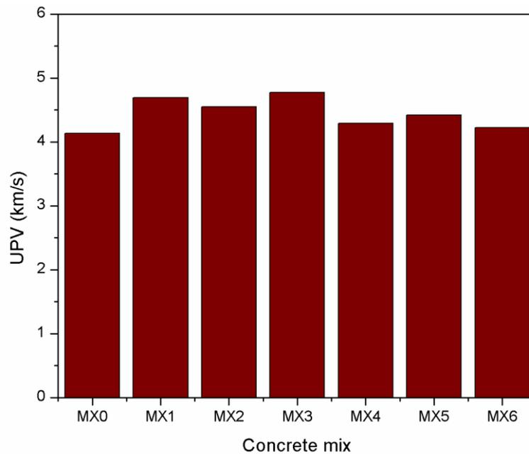
Fig. 4 Ultrasonic pulse wave of concrete at the curing ages of 28 days
