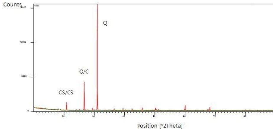
Fig. 7 X-Ray Diffraction of MX0 at the curing ages of 28 days (Q = quartz; CS = calcium silicate; CSH = calcium silicate hydrate)
