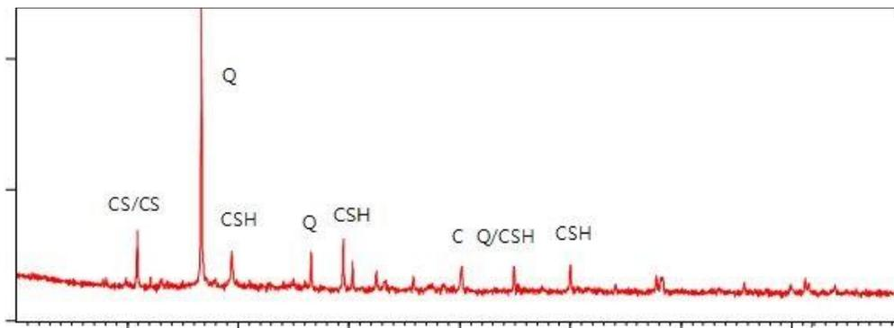
Fig. 8 X-Ray Diffraction of MX1 at the curing ages of 28 days (Q = quartz; CS = calcium silicate; C = calcite; CSH = calcium silicate hydrate)
