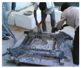
Fig. 2 Specimens concreting and vibrating
