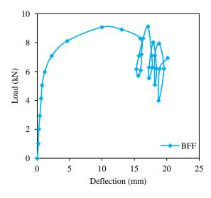
Fig. 7 Load - displacement profile of BFF specimens
