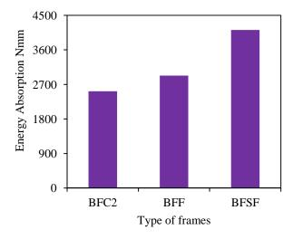
Fig. 10 Comparison of energy absorption by ductile and non-ductile frames
