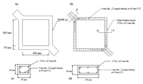
Fig. 1 Schematics of (a) mould (b) reinforcement (c) cross section AA and (d) cross section BB
