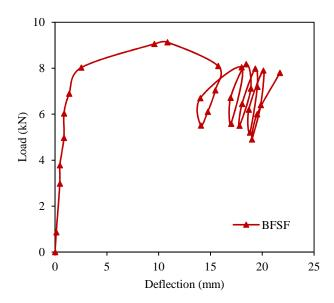
Fig. 9 Load - displacement profile of BFF specimens
