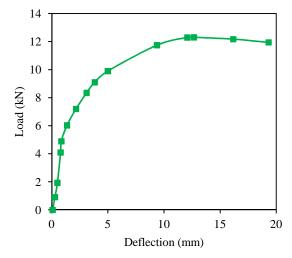
Fig. 4 Load-displacement profile of BFC1 specimens
