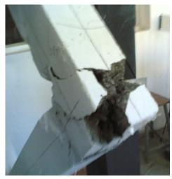
Fig. 8 Typical plastic hinge pattern
