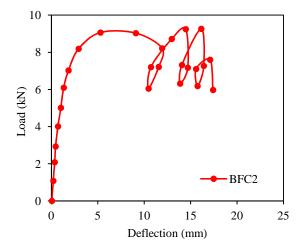
Fig. 5 Load-displacement profile of BFC2 specimens
