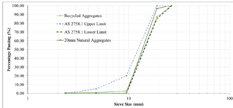
Fig. 2 Sieve analysis of recycled coarse aggregates and natural coarse aggregates.
