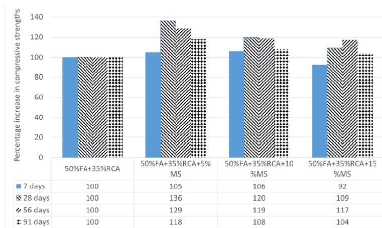
Fig. 5 Percentage changes in the compressive strength of HVFA-RAC relative to concrete in series 2 due to addition of MS
