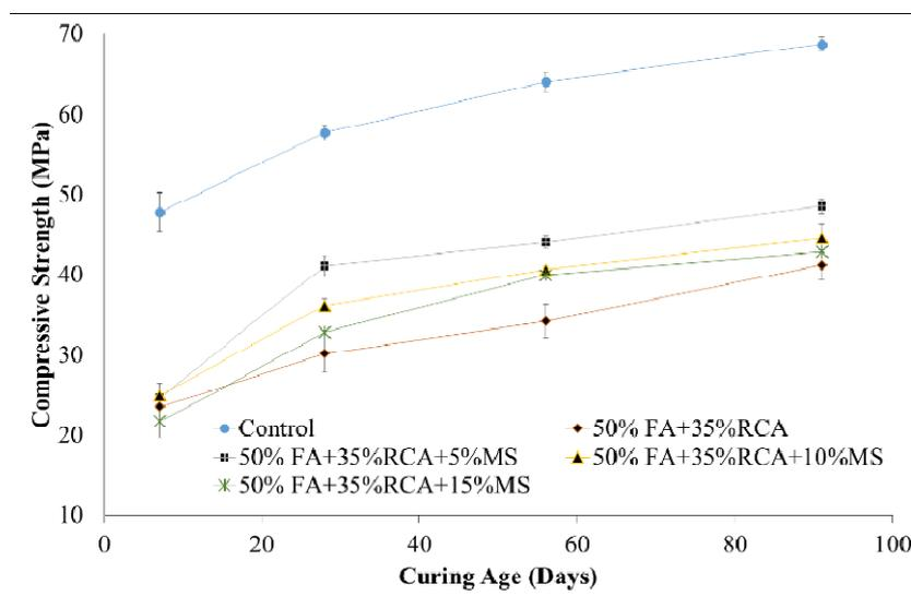
Fig. 4 Effects of MS on the compressive strength of high volume fly ash recycled aggregate concretes
