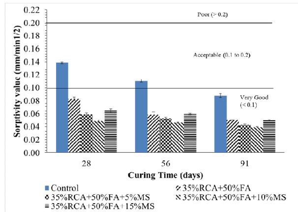
Fig. 12 Effect of MS on water sorptivity of HVFA-RAC
