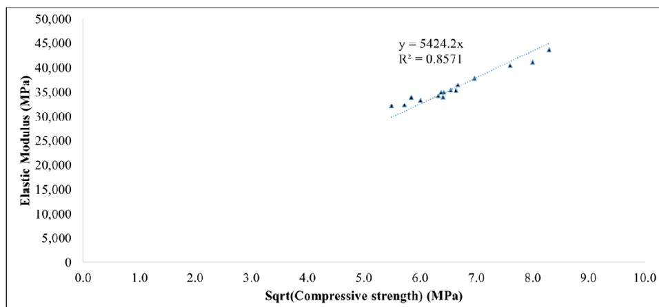
Fig. 10 Correlation of elastic modulus with compressive strengths
