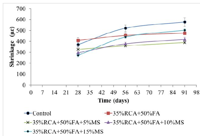
Fig. 14 Effect of MS on drying shrinkage of HVFA-RAC
