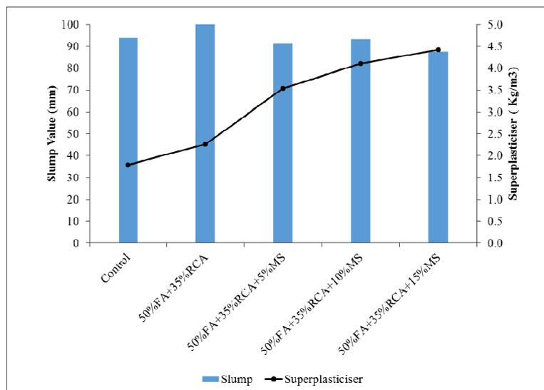
Fig. 3 Workability of concretes
