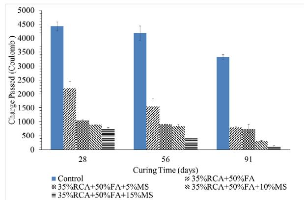
Fig. 13 Effect of MS on chloride ion permeability of HVFA-RAC
