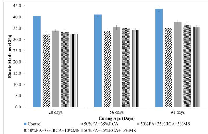
Fig. 9 Effects of MS on elastic modulus of high volume fly ash recycled aggregate concretes
