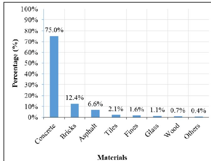
Fig. 1 Contents analysis of recycled coarse aggregates
