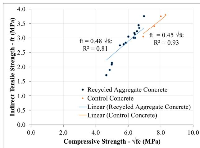
Fig. 8 Correlation of indirect tensile strengths with compressive strengths
