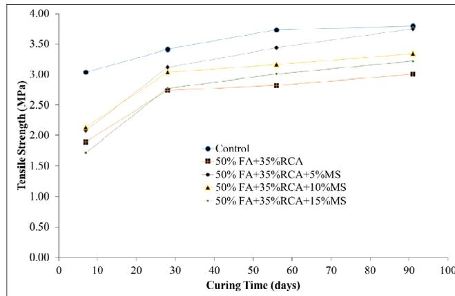
Fig. 6 Effects of MS on the indirect tensile strengths of high volume fly ash recycled aggregate concretes
