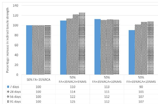
Fig. 7 Percentage changes in the indirect tensile strength of HVFA-RAC relative to concrete in series 2 due to addition of MS
