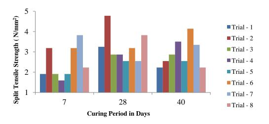
Fig. 5 Variation in split tensile strength with curing period
