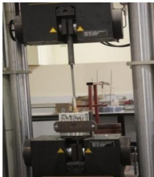
Fig. 3 Experimental pullout test setup using a UTM with 1200 kN load capacity
