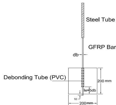
Fig. 1 Geometric description of the pullout sample
