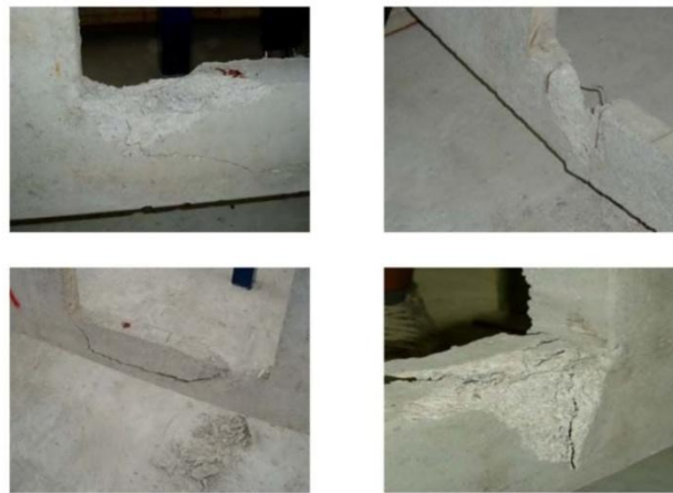
Fig. 15 Photographs of some beams after failure
