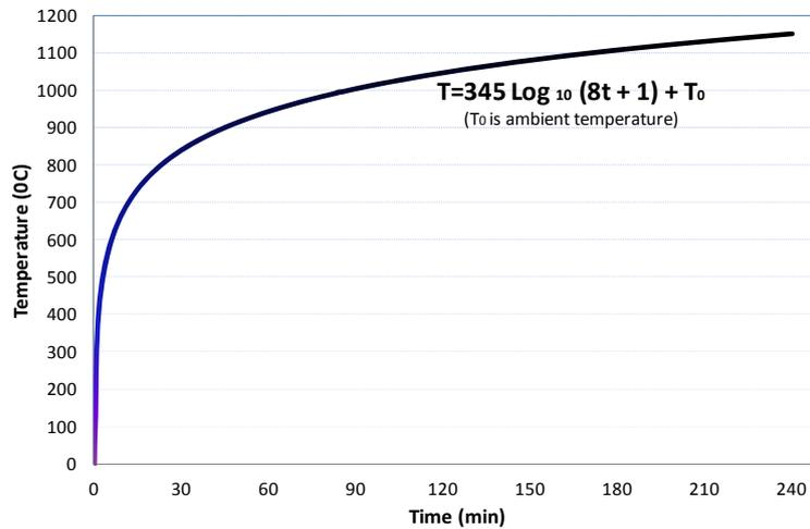
Fig. 8 Fire pattern according to ISO834
