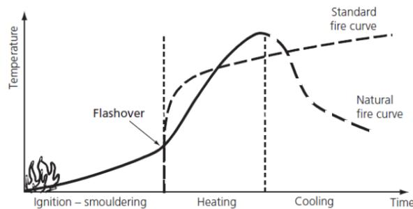
Fig. 7 Temperature-time curve for fully developed fire (Lennon 2011)
