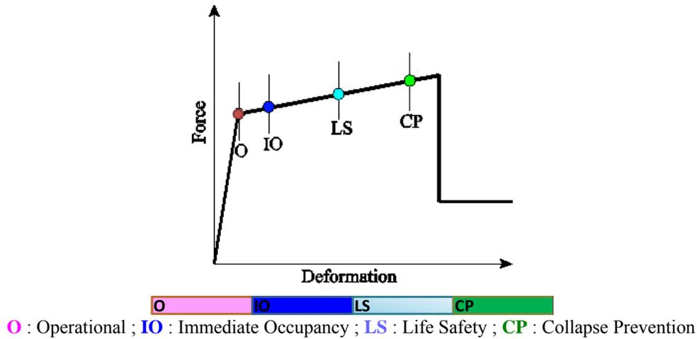
Fig. 4 Conceptual plastic hinge states
