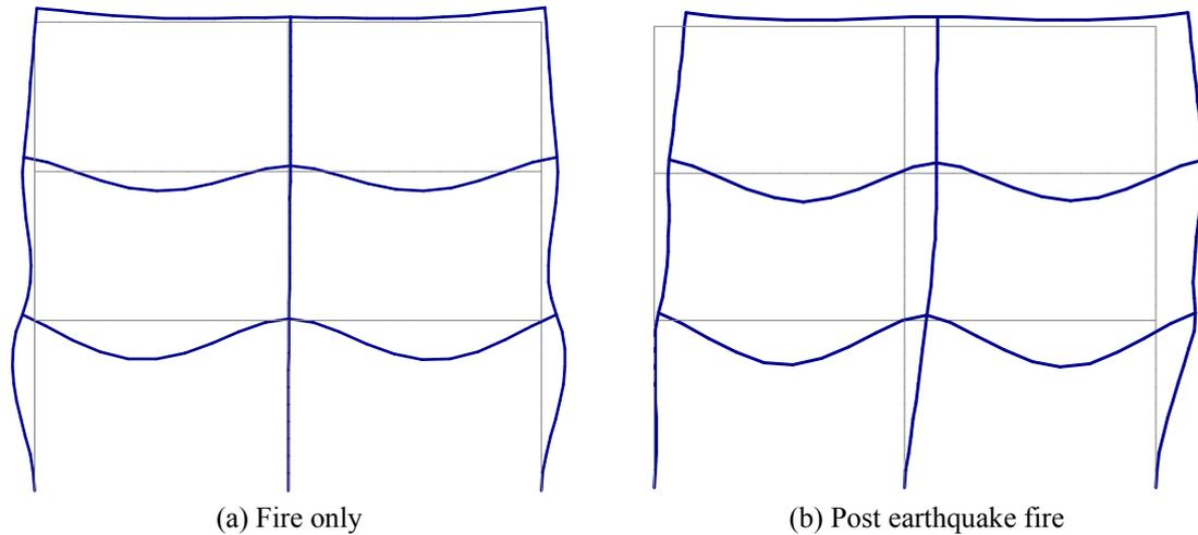
Fig. 15 Collapse mechanism for the models, before and after earthquake
