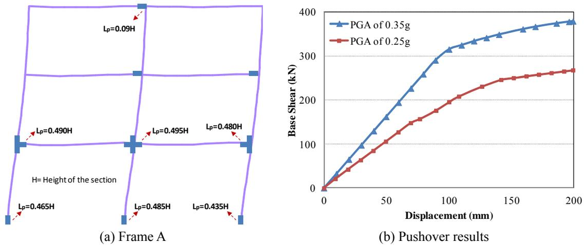
Fig. 11 Extend of plastic hinges in Frame A and pushover curves in Frame A and B
