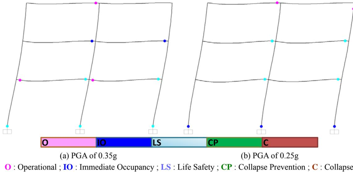
Fig. 10 Plastic hinges states of the structures resulted from pushover analysis
