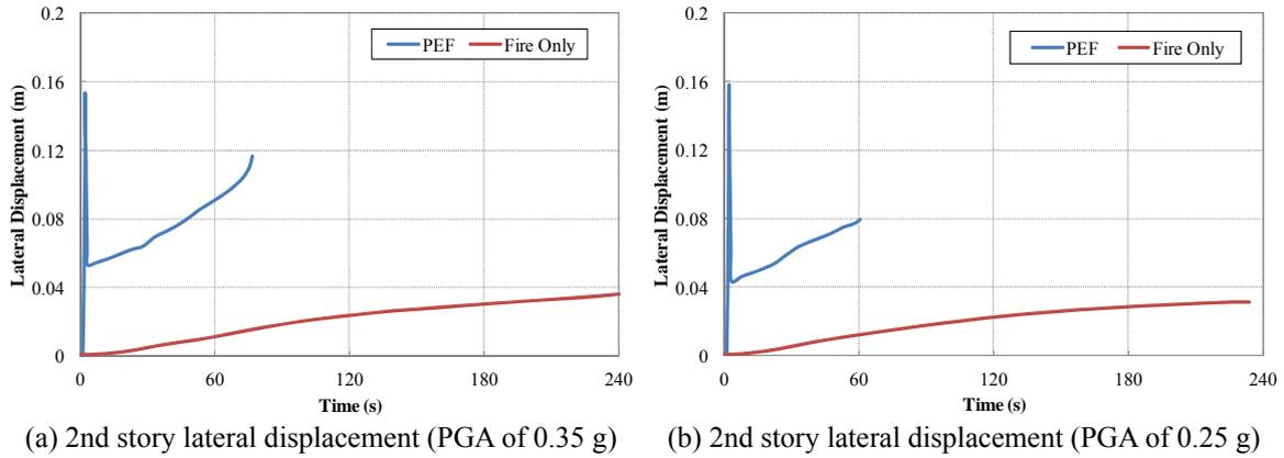
Fig. 13 Fire resistance based on scenario 1 (fire initiated from first and second floors)
