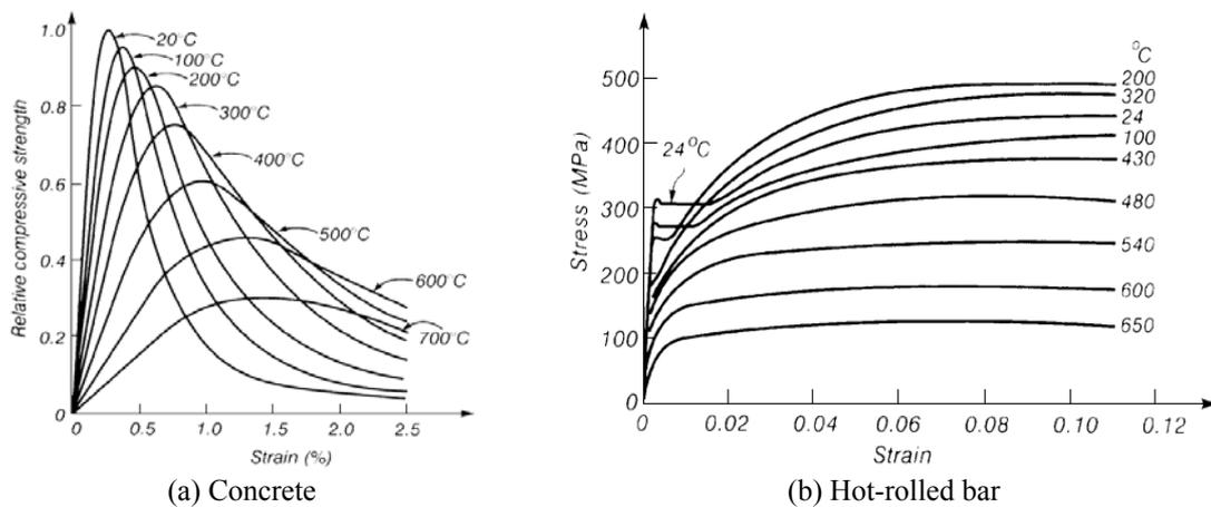
Fig. 6 Stress-strain relationship at different temperature (Minson 2006)
