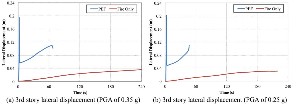
Fig. 14 Fire resistance based on scenario 2 (fire initiated from second and third floors)
