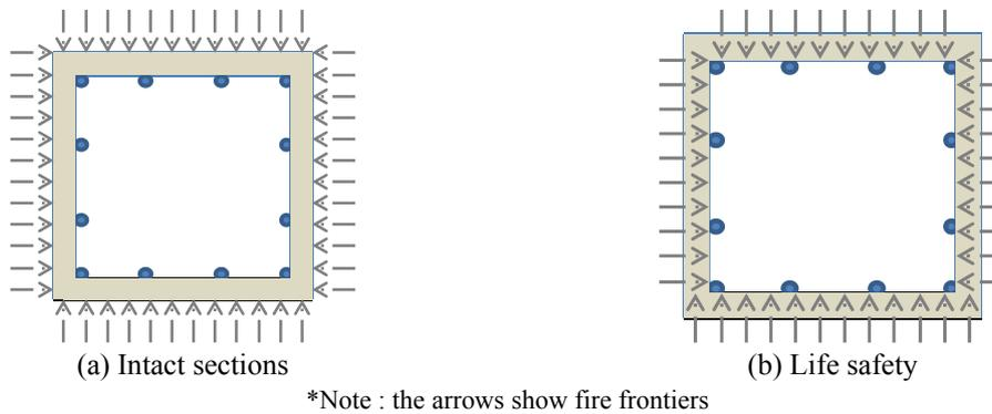
Fig. 5 Applied fire frontiers on the damaged sections
