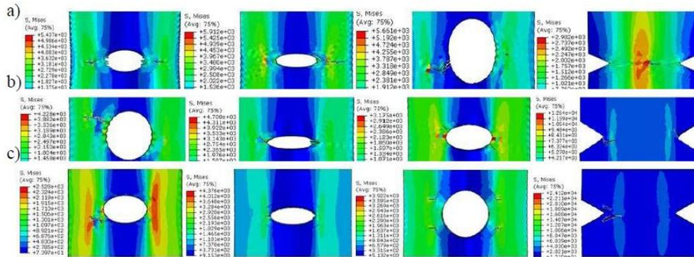
Fig. 9 Stress distribution of each form of notch under (a) modification1 and (b) modification 2 (c) modification3
