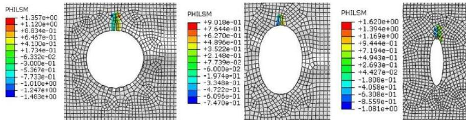
Fig. 10 Contours of PHILSM of the XFEM technique
