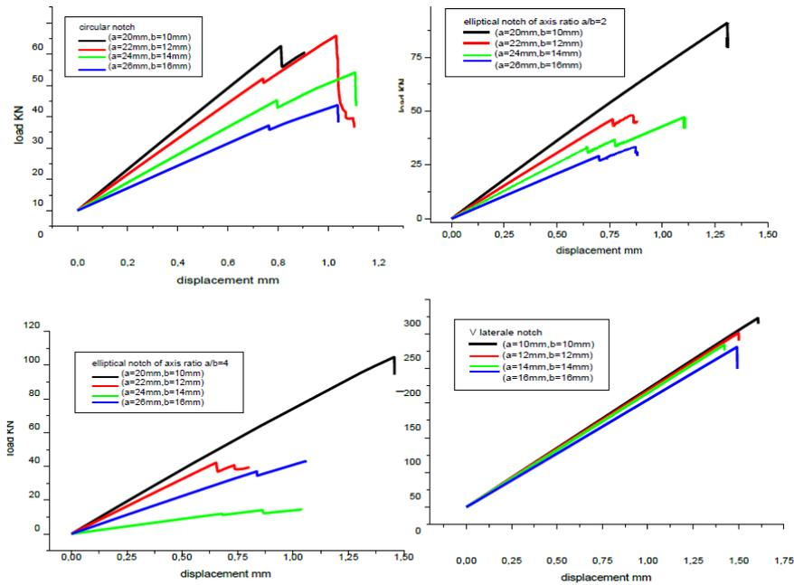
Fig. 5 XFEM load displacement curve of (a) circular, (b) elliptical of  $a/b=2$  and (c) elliptical of  $a/b=4$  and (d) lateral V, for different deferent notch size
