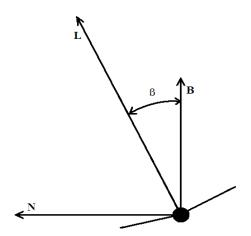
Fig. 2 The angle of bank in relation to the unit vectors N and B
