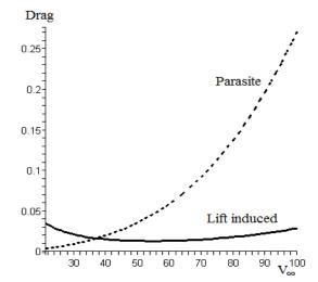
Fig. 7 Llift induced drag (full line) and parasite drag (dotted line) for the Cessna 182
