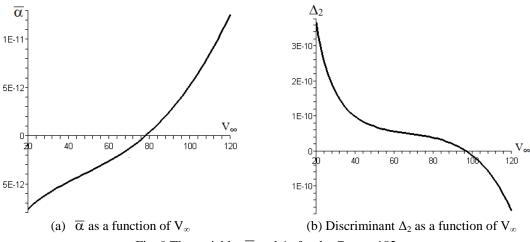
Fig. 9 The variables  $\overline{\alpha}$  and  $\Delta_2$  for the Cessna 182
