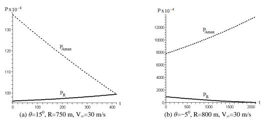
Fig. 5 Power required  $P_R$  (solid line) and the maximum power available  $P_{Amax}$  (dotted line), for the Cessna 182
