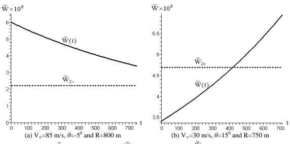
Fig. 11  $\widetilde{W}(t)$  and its lower bound  $\widetilde{W}_{2-}$  and its upper bound  $\widetilde{W}_{2+}$ , for the Cessna 182
