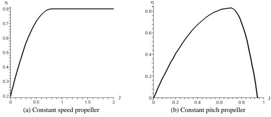
Fig. 12 Typical efficiency factor as a function of the advance ratio J
