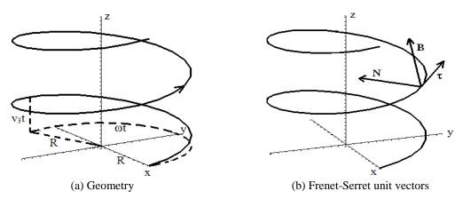
Fig. 1 Ascending helical trajectory
