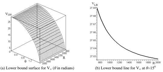
Fig. 3 Bound on the speed  $V_{\infty}$  due to the bound on the lift coefficient for the Cessna 182
