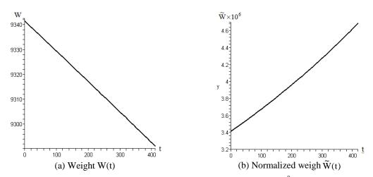
Fig. 4 Weight variation in time for a Cessna 182 ascending on a helix with  $\theta$ =15<sup>0</sup>, R=750 m and V<sub>∞</sub>=30 m/s
