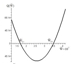
Fig. 8 Q( $\widetilde{W}$ ) in terms of  $\widetilde{W}$ , for the Cessna 182, with V<sub> $\infty$ </sub>=30 m/s, =-5<sup>0</sup> and R=800 m
