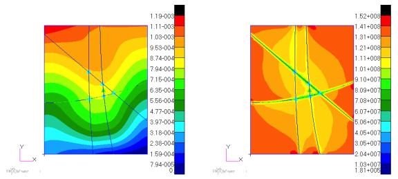
Fig. 11 Pylon wing panel,  $0.4064 \text{ m} \times 0.5080 \text{ m}$ , four stiffeners, optimization using QNSTOPS: (a) displacement (m), and (b) von Mises stress distribution (Pa)
