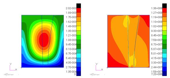
Fig. 7 Pylon wing panel,  $0.4064 \text{ m} \times 0.5080 \text{ m}$ , two stiffeners, optimization using VTdirect: (a) displacement (m), and (b) von Mises stress distribution (Pa)
