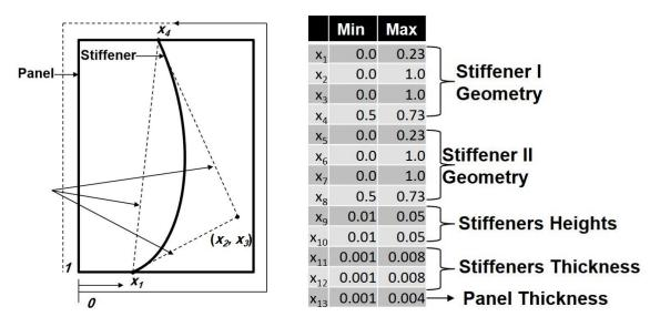
Fig. 2 Design variables of the stiffener (left). Definition and range of the design variables for the optimization process (right)
