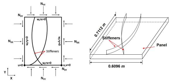
Fig. 4 Curvilinear stiffened panels under combined shear and normal loads
