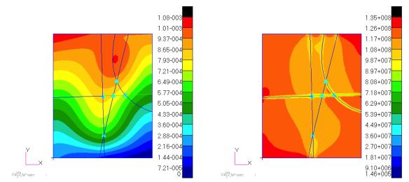
Fig. 10 Pylon wing panel,  $0.4064 \text{ m} \times 0.5080 \text{ m}$ , four stiffeners, optimization using VTdirect: (a) displacement (m), and (b) von Mises stress distribution (Pa)
