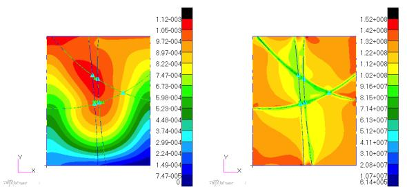
Fig. 12 Pylon wing panel,  $0.4064 \text{ m} \times 0.5080 \text{ m}$ , four stiffeners, optimization using QNSTOPP: (a) displacement (m), and (b) von Mises stress distribution (Pa)
