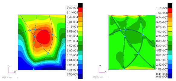
Fig. 5 Pylon wing panel, 0.6096  $m \times 0.7112$  m, four stiffeners, optimization using pVTdirect: (a) displacement (m), and (b) von Mises stress distribution (Pa)
