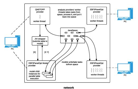
Fig. 3a Use of JavaSpaces technology (a) and Catalog technology (b) in a dynamic distributed computing environment for the panel optimization studies
