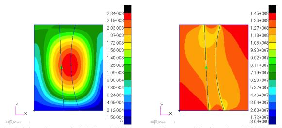
Fig. 9 Pylon wing panel,  $0.4064 \text{ m} \times 0.5080 \text{ m}$ , two stiffeners, optimization using QNSTOPP: (a) displacement (m), and (b) von Mises stress distribution (Pa)
