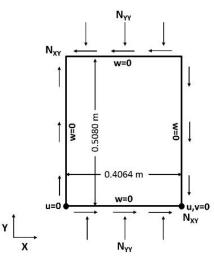
Fig. 6 Conventional aircraft wing panel geometry along with the loads
