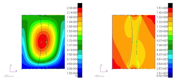
Fig. 8 Pylon wing panel,  $0.4064 \text{ m} \times 0.5080 \text{ m}$ , two stiffeners, optimization using QNSTOPS: (a) displacement (m), and (b) von Mises stress distribution (Pa)
