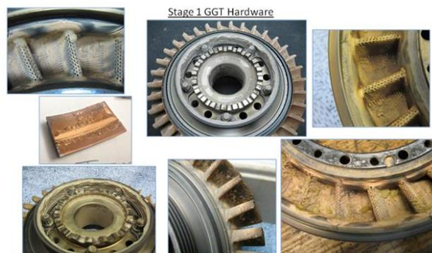
Fig. 4 Sand glazing deposits found on Gas Generator Turbine (GGT) hardware from field returned engines
