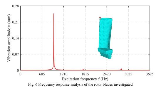
are identified where natural frequencies of the blade and the EO line coincides. In this particular example, the resonance points are at frequencies of 929.56, 1752.92 and 2818.28 Hz.
