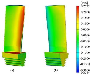
Fig. 1 Evaluated deviations between measured and ideal geometry of one turbine blade using GOM Inspect viewed (a) from the front and (b) from the back
