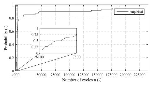
Fig. 14 Variance in lifetime caused by variable material parameters
