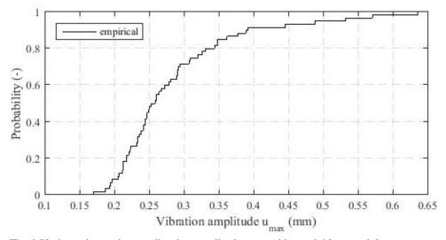
Fig. 9 Variance in maximum vibration amplitudes caused by variable material parameters
