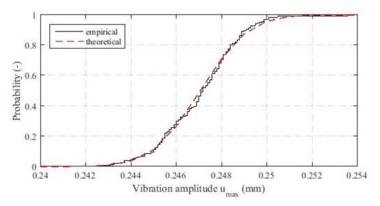
Fig. 8 Variance in maximum vibration amplitudes caused by variable geometrical parameters
