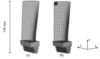
Fig. 3 Finite element mesh of the turbine blade investigated (a) without repair and (b) with patch
