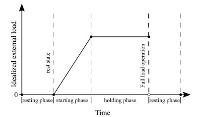
Fig. 4 Computation cycle for one flight operation
