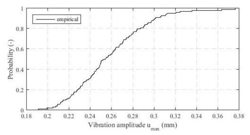
Fig. 10 Variance in maximum vibration amplitudes caused by variable material parameters of the patch
