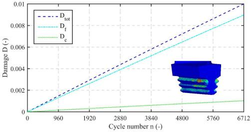
Fig. 12 Maximum local damage within the rotor blades
