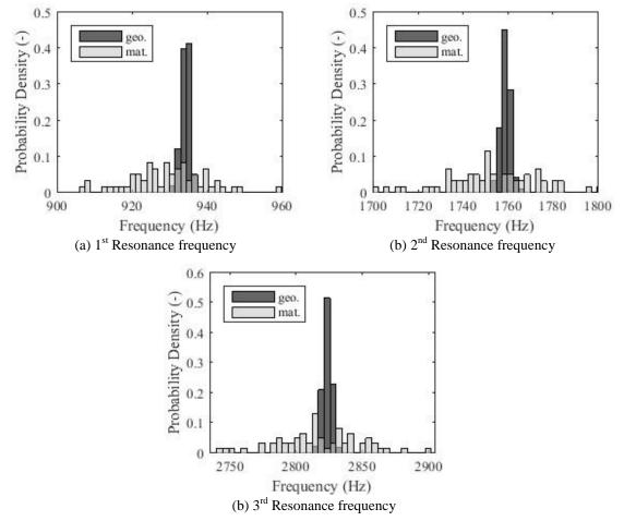
Fig. 7 Scatter of resonance conditions due to scatter in geometrical (geo.) and material (mat.) parameters
