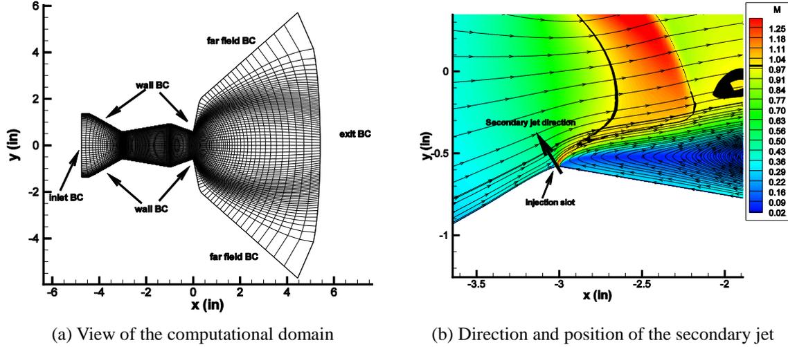
Fig. 2 Dual throat nozzle computational domain and boundary conditions
