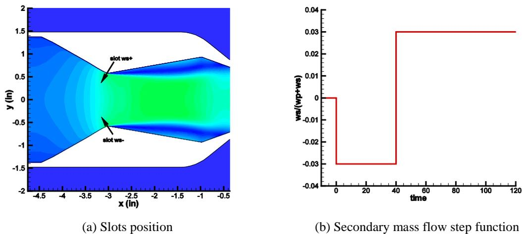
Fig. 8 Slots position and mass flow function for unsteady simulation at NPR=4
