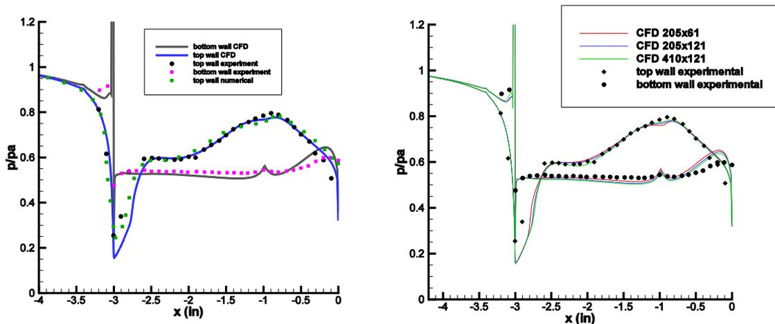
(a) Static pressure comparison (b) Static pressure on different meshes
