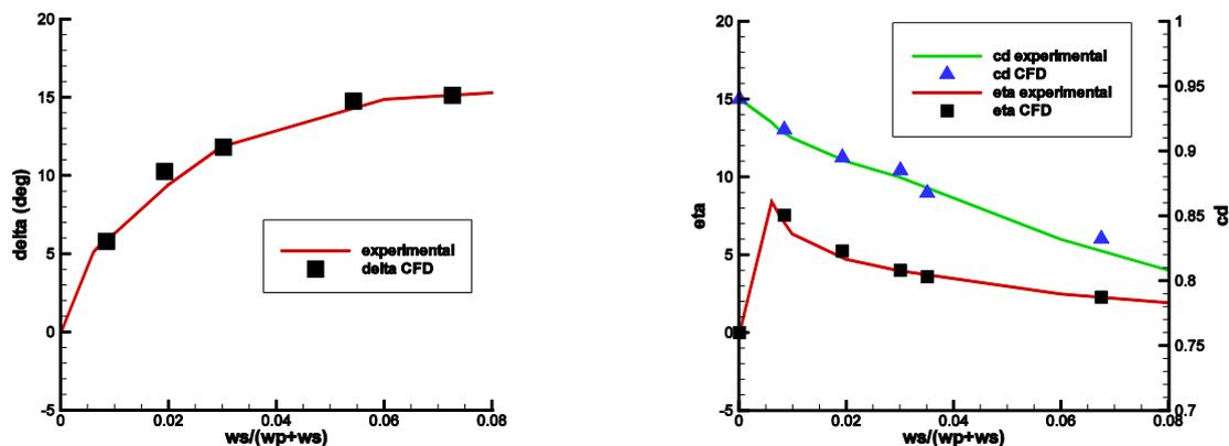
(a) Pitch thrust angle,  $\delta_p$ , comparison(b) Discharge coefficient,  $C_d$ , and thrust vectoring efficiency,  $\eta$ , comparison
