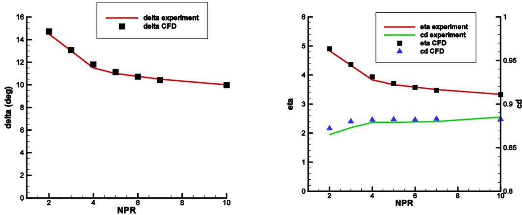
(a) Pitch thrust angle,  $\delta_p$ , 3% injection(b) Discharge coefficient,  $C_d$ , and thrust vectoring efficiency,  $\eta$ , 3% injection
