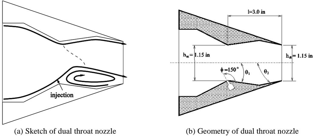
Fig. 1 Dual throat fluidic thrust vectoring nozzle
