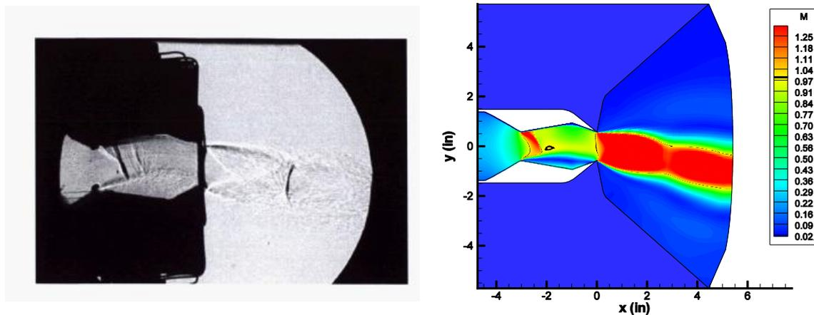
(a) Experimental shadowgraph (Flamm *et al.* 2006) (b) Numerical Mach contour lines
