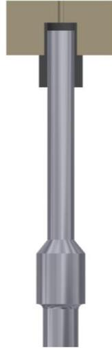
Fig. 3 Scheme of the microphone cavity and the pinhole. The microphone is mounted through a properly designed connector. The pinhole diameter is 1.5 mm
