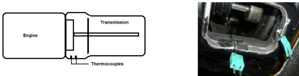
(a) The thermocouples on engine transmission assembly (b) The thermocouples in the clutch housing
