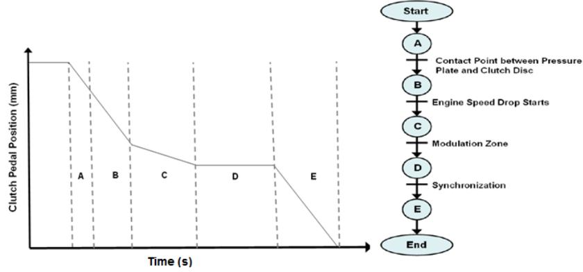
Fig. 5 Theoretical clutch pedal position during drive-off
