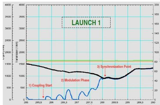
Fig. 19 Angular speeds of engine flywheel and transmission input shaft at 1<sup>st</sup> drive-off
