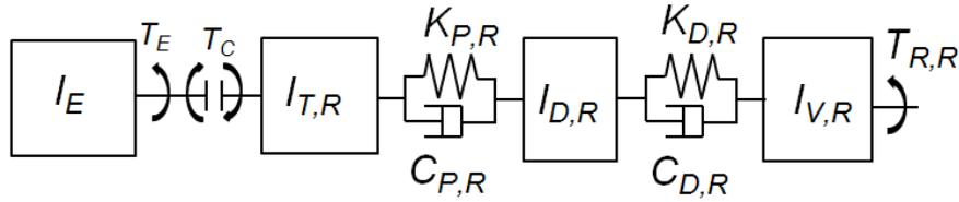
Fig. 3 Simplified model of the driveline
