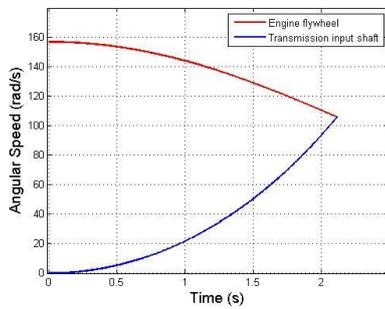
(a) The angular velocities of the engine flywheel and the transmission input shaft
