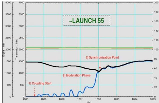
Fig. 21 Angular speeds of engine flywheel and transmission input shaft at 55<sup>th</sup> drive-off
