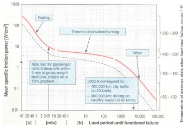
Fig. 15 The effect of mean friction power on the total clutch life (Coelho and Rabelo 2011)
