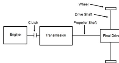
Fig. 1 Heavy duty vehicle driveline
