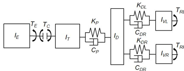
Fig. 2 Model of the driveline
