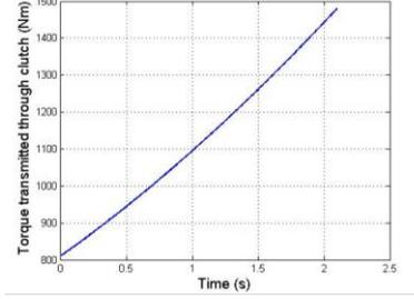
(b) The torque transmitted through the clutch
