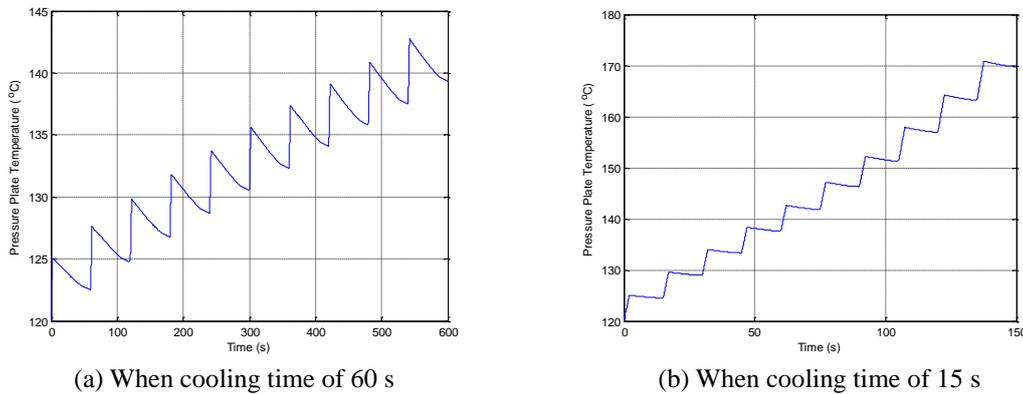
Fig. 16 Temperature of pressure plate during drive-off when the pedal travels with the same speed all the way in modulation zone
