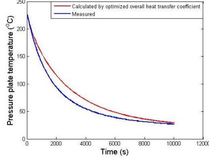
Fig. 11 Comparison of calculated by cooling model and experimentally measured pressure plate temperature
