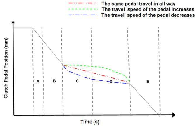
Fig. 6 Driver profiles for clutch pedal travel during slip time
